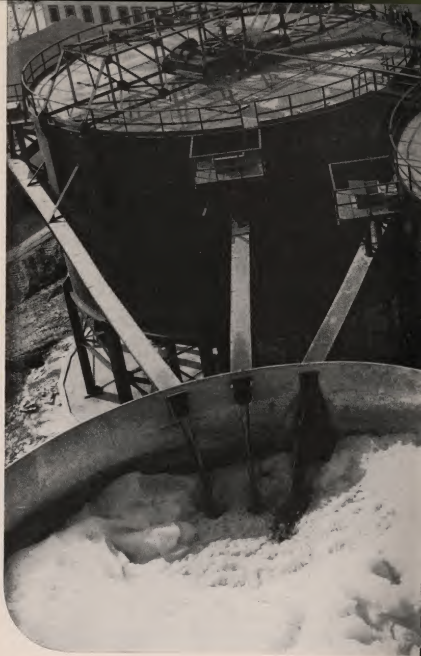
A step in the wet chemical process for obtaining alumina, or aluminum oxide, from bauxite. The alumina is later reduced to aluminum.
